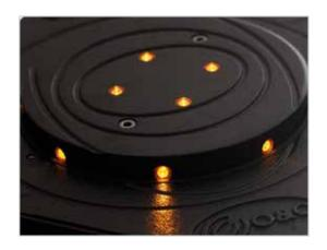
This heavy duty product is developed for the protection and defence of sensitive and/or strategic sites such as prestigious buildings, hotels etc. K12 rated in accordance to ASTM2656:2007 M50 including PAS68:2010 7500/80/N3 AND IWA14-1:2013 V/7200[N3C]/80/90. Each bollard can be fitted with a 100mm wide reflective strip and is available in blue grey (RAL 7031). Designed for lowering functionality after impact. This bollard has Interfaces for remote control.
